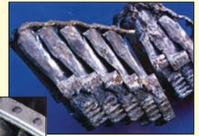
Turbine Blade Damage Due to Water Carry Over in Steam Supply
