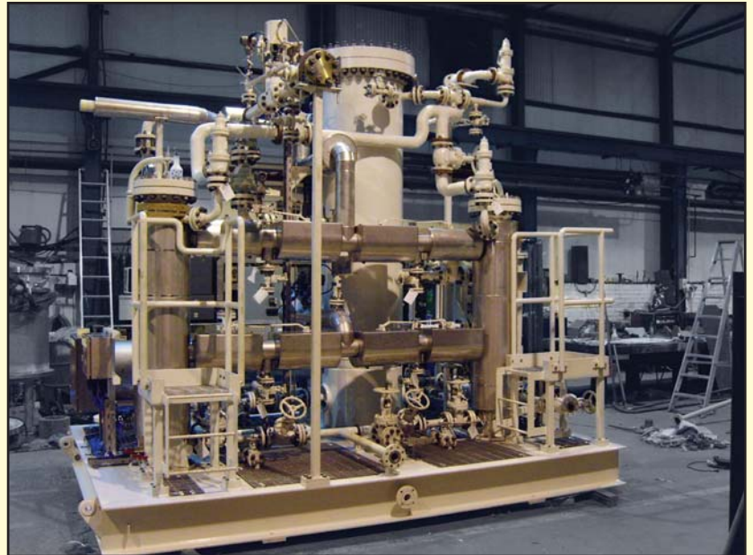
Fuel Gas Conditioning Skid
